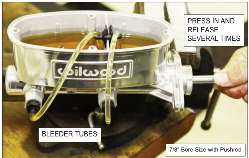
Typical Bleeder Tube Setup and Use
